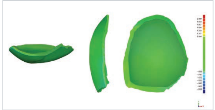
A deviation map is generated from the white light data and compares the STL design file to the final manufactured implant.
